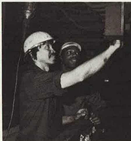
Car Inspectors Ernie Martin (left) and Mike Lindsay (right) change the pressure switch while working under an R46.
