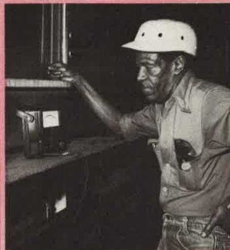
On an R46, Charlie Barker checks the converter/inverter.
